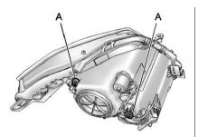
For the vehicle equipped with an up-level headlamp (HID), there will be two vertical headlamp adjusters (V1 and V2).
